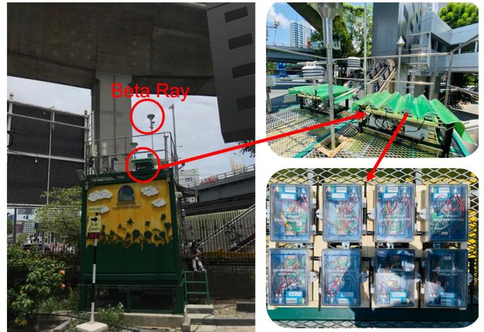
Figure 3: The Canarin nodes were tested in an ambient environment by co-locating with a Beta Ray air quality station
